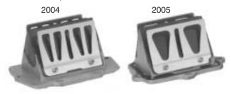
Revised intake manifold provides a straighter path to the engine for improved throttle response.
